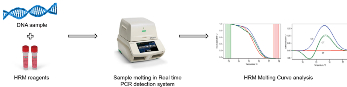
Figure 8. HRM workflow. Adapted from Bio-Rad ( http://www.bio-rad.com ).
