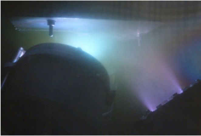
Figure 5.33: FFE75 full face erosion magnetron (left) and IMC75 Ion Source (right) in operation.
