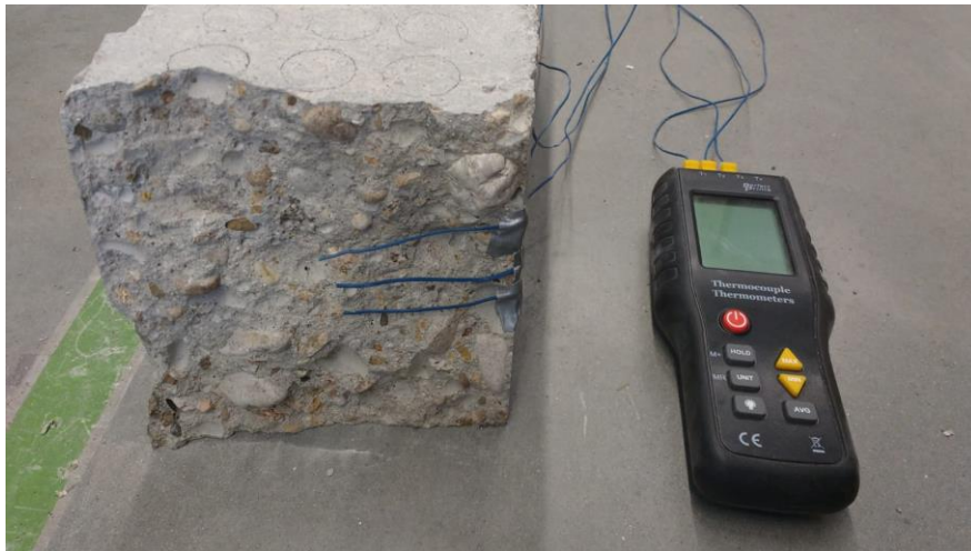
Figure 8: Thermocouples on specimen
