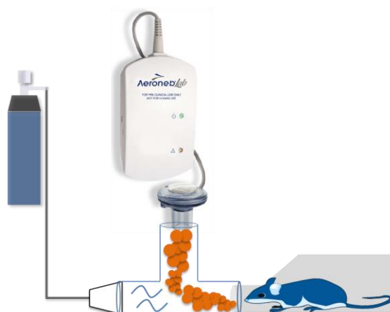
Figure 4.3. Illustration of the Aeroneb Lab Micropump Nebulizer connected to the rat holder.
