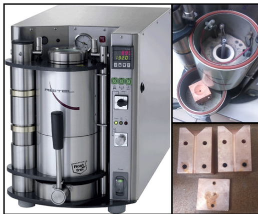
Figure A.1: (Left) Reitel Induret Compact induction furnace used for master alloys production (Right) Crucible and copper mold are utilized for melting and casting.
