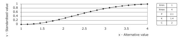
*Figure 33: Shape, tendency and maximum and minimum satisfaction values of the "drainage system condition" indicator. Source: Author*
