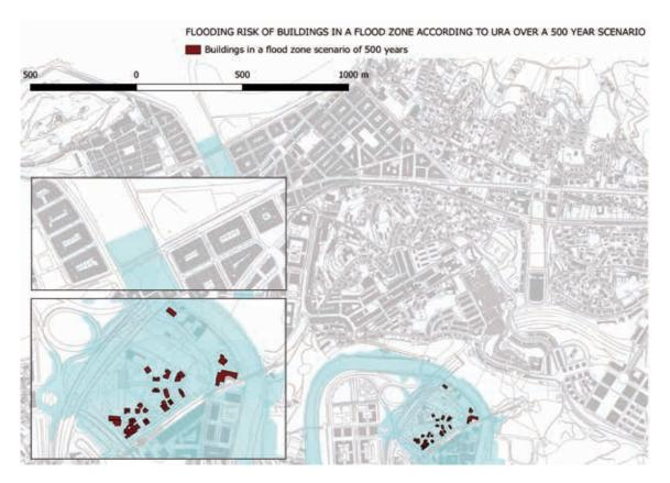
Figure 42: Flooding in a 500 year scenario in the case study area of San Sebastian. Source: Tecnalia
