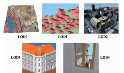
Figure 10: The five levels of detail (LoD) defined by CityGML. Source: (Kolbe 2009)
