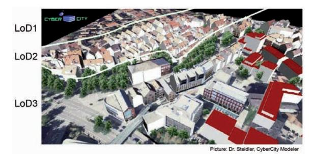
*Figure 11: Different Levels of Detail in a scene. Source: http://www.directionsmag.com/entry/citygml-an-open-standard-for-3d-city-models/123103*
