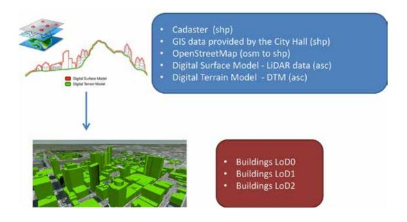
Figure 53: Geometric generation of 3D urban model. Source: Tecnalia
