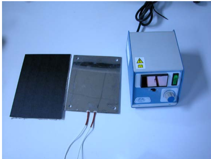
Figure A5.1: Heat power source for the test bench
