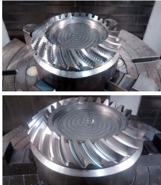
Figure 13. Gear after rough ( top ) and finish machining ( bottom ).
