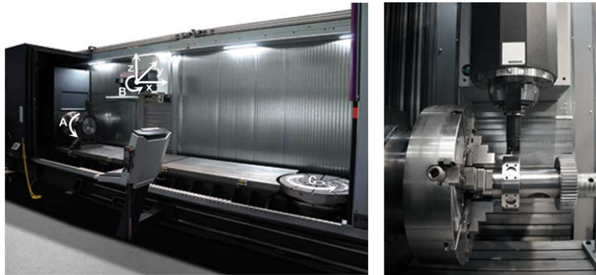
Figure 5. Ibarma multiprocess machine ZVH38/L1600 (left), Ibarma ZVH38/L1600 A axis and head (right).
