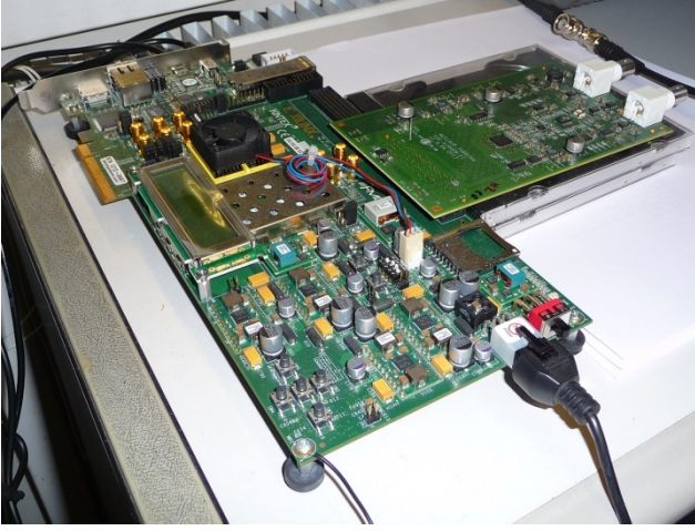
Fig. 3 Analog front-end card plugged into the KC705 development card
