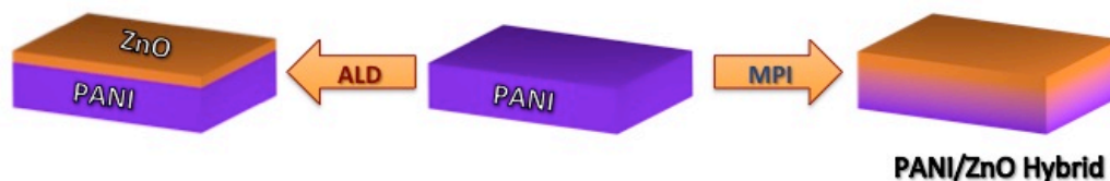
Figure 5.1 Schematic indicating the different resulting types of composites once a polymer is processed by atomic layer deposition (ALD) or multiple pulsed vapor phase infiltration (MPI). With MPI the substrate is exposed to vapors of DEZ and H 2 O in a sequential manner. Extended exposure times enable the precursors to diffuse into the polymer and react with the molecular backbone in the subsurface area forming a polymer-inorganic hybrid with a concentration gradient depending on the duration of exposure.
