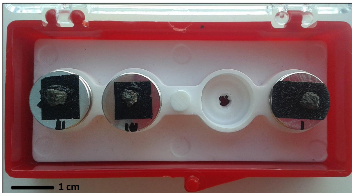
Figure 3.2. Fragments of the initial NWA 6148 sample attached to pins with carbon adhesive tape.
