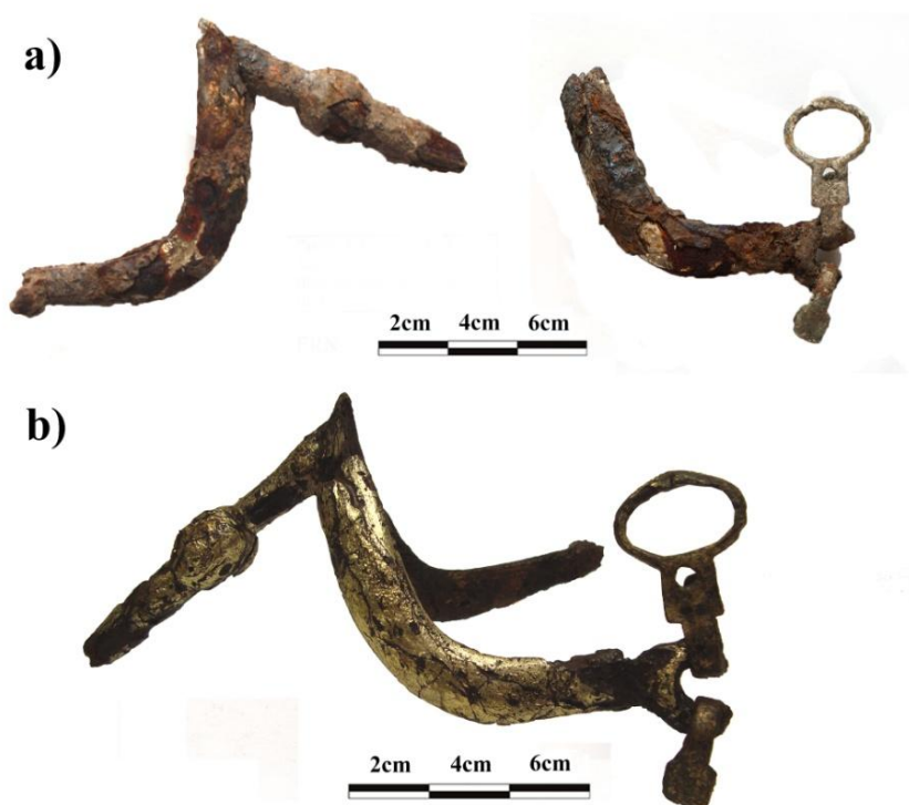
Figure 6.6: Middle Age gilded spur proceeding from the Ereñozar necropolis before (a) and after (b) restoration. The conservation treatments applied by restorers included desalination, consolidation and removal of the outer corrosion layers.
