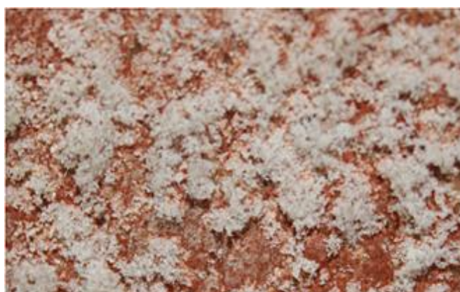
Figure 1.9: Mural painting from the archaeological site of Pompeii (Italy) showing critical damages due to soluble salt crystallization (source: J.M. Madariaga et al. (2014) [104]).
