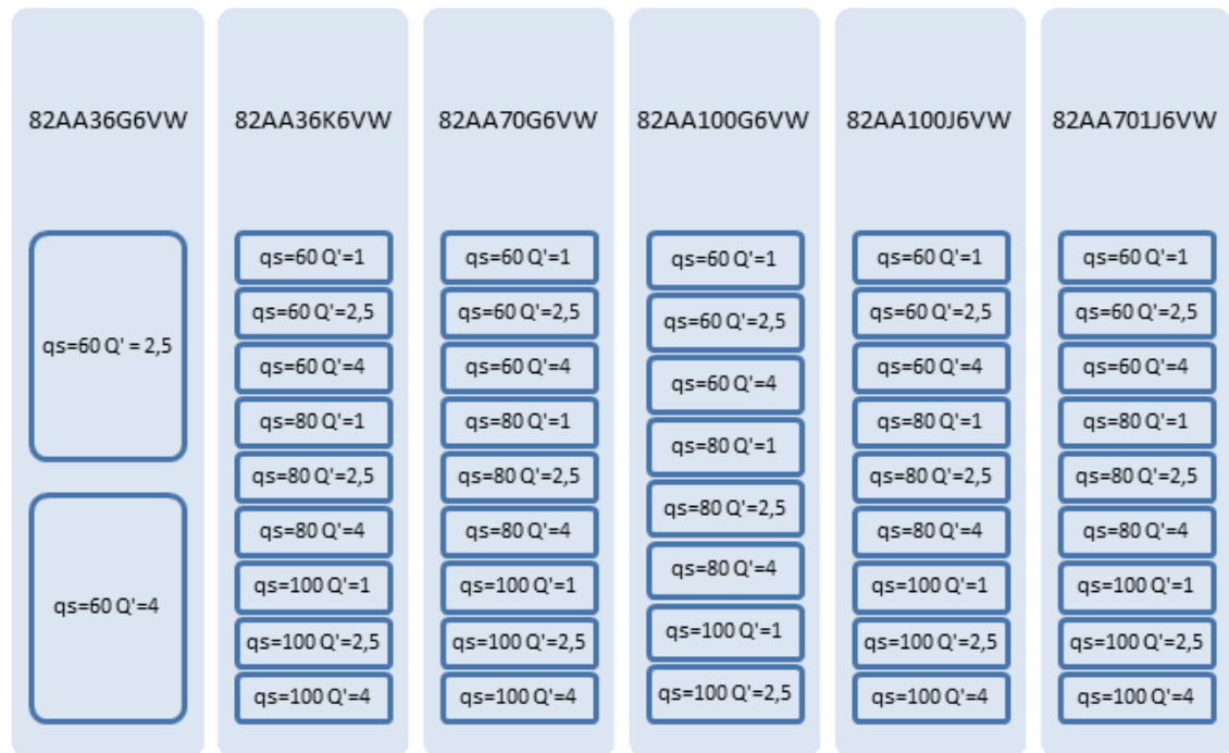
Figure 21 Grinding wheels and grinding conditions used to carry out the experiments to generate the training database
