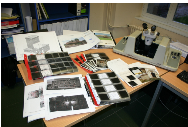
Figure 2. Display of a stereoplottor for analog photographs, Adam MSP-2 (at present, out of order), together with several folders with 6x6 cm negatives of some projects, plans, sketches with the distribution of the control points, complementary photographs, etc. The description of the analog equipment (e.g. cameras or stereoplotters) can be found in reference texts of that time (such as Atkinson, 1989).
