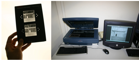
Figure 3. Slide holder for 6x6 cm analog negatives (left) and scanning device employed (right).
