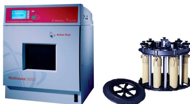
Figure 3.18. Multiwave 3000 microwave (Anton Paar, Graz, Austria) and Teflon vessels for digestion.
