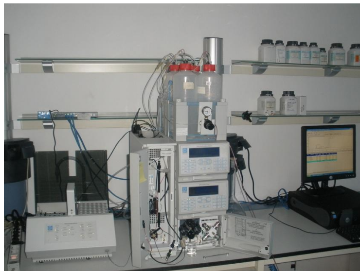
Figure 3.17. Ion chromatograph coupled to a conductimetric detector with postcolumn suppression and AS 40 autosampler (Dionex).
