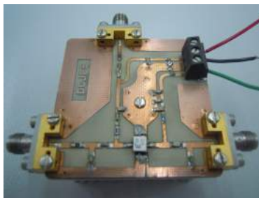
Figure 2.15: Photography of the medium power FET amplifier in L band.
