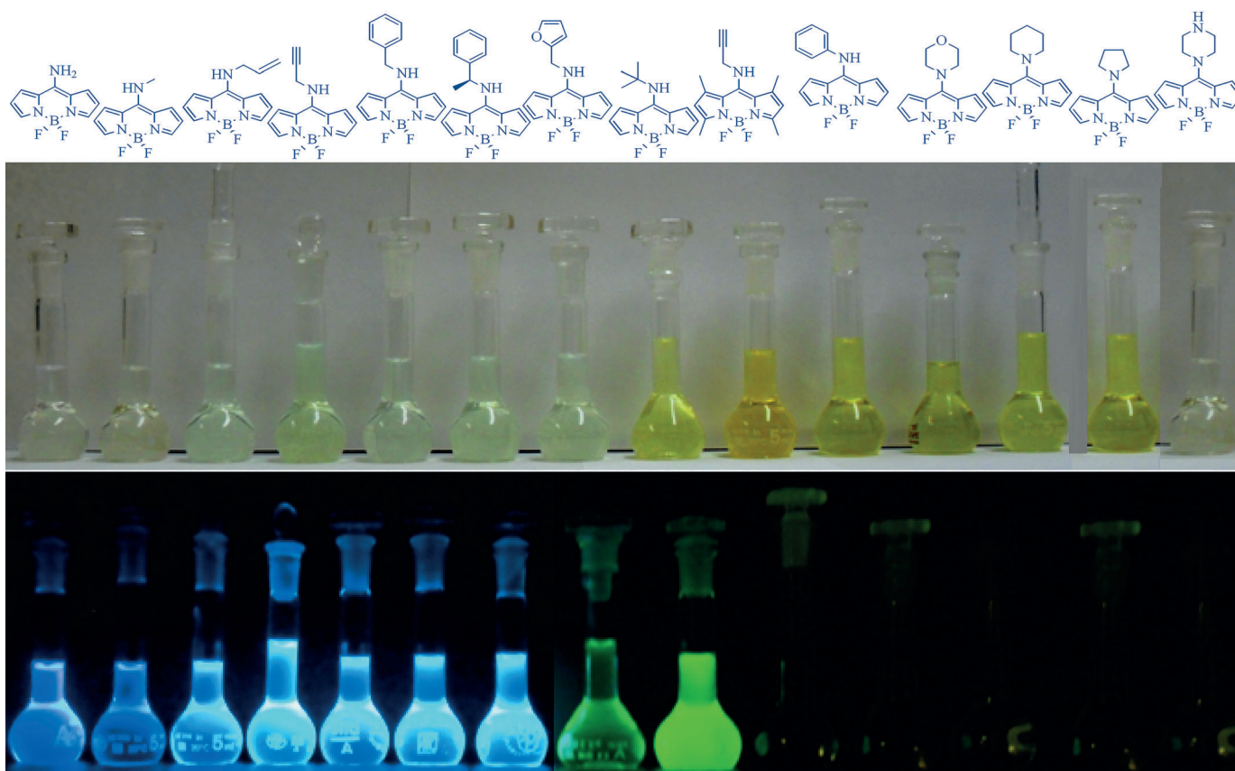
Figure 6. Fluorescent response of the 8-aminoBODIPY dyes to the nature of the amino group (solutions in ethyl acetate, under excitation at \lambda = 366 nm).
