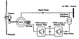
Figure 1. Scheme of a DFIG equipped wind turbine
