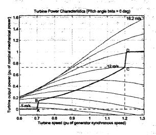
Figure 2. Turbine Power Characteristics
