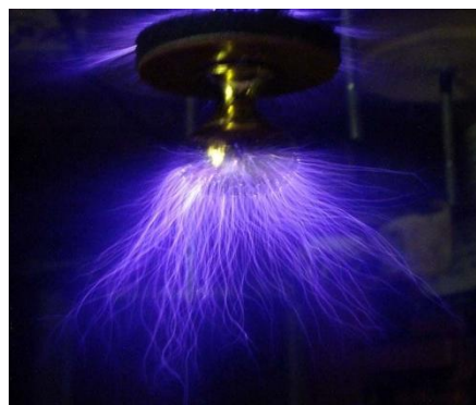
Figure 3.3. Photography of a corona discharge.
