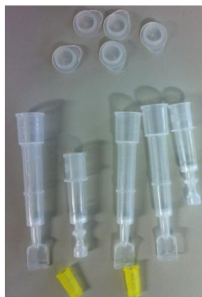
Figure 2.12. Bio-spin chromatography columns from Bio-Rad used during the SELEX procedure.
