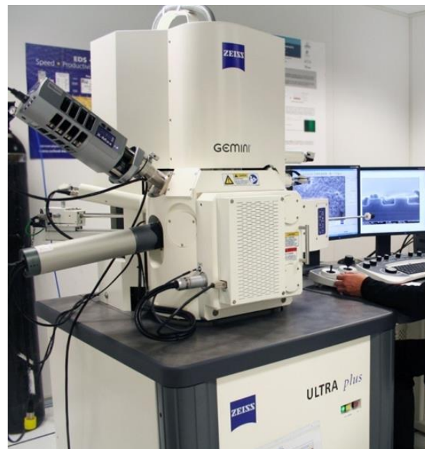
Fig 3. 6: FE-SEM microscope used for TaN x films analysis
