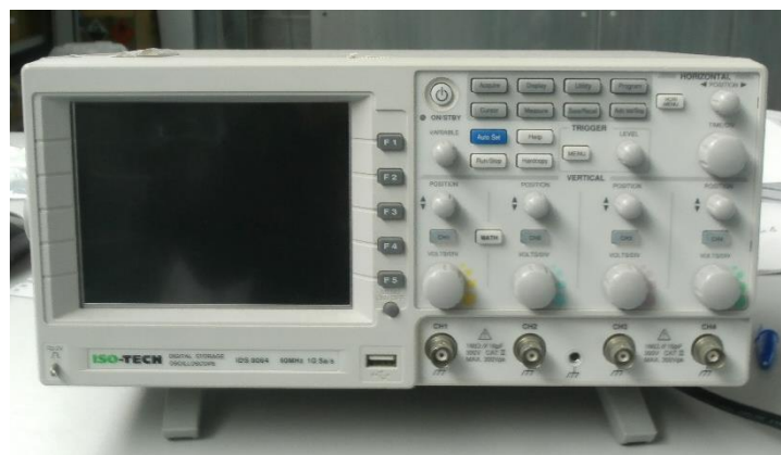
Fig 3. 3: ISO-TECH oscilloscope employed for V-I waveforms monitoring
