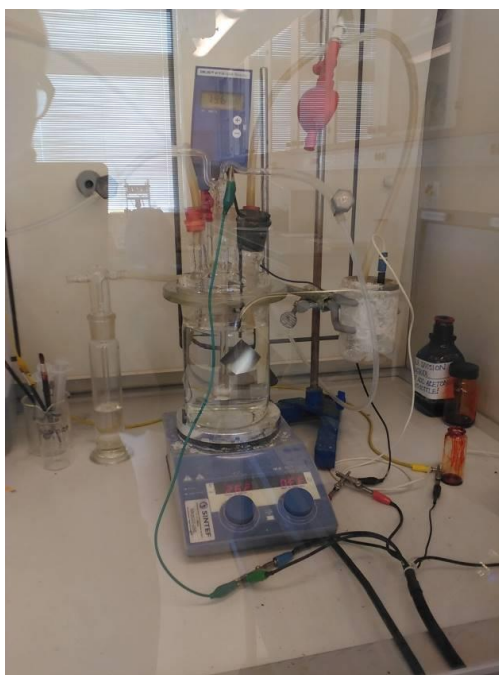
Fig 6. 4: Electrochemical set-up for ex-situ testing of TaN x coated SS316L in PEMFC environment
