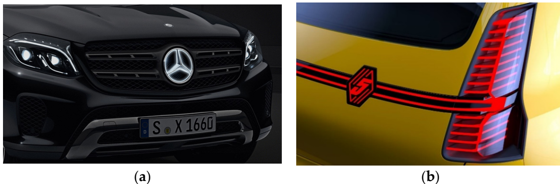
Figure 4. This figure shows how decorations are being upgraded with electronic components, such as LED illumination: (a) illuminated badge on a 2016 Mercedes-Benz GLE (W166); (b) illuminated rear badge on the next Renault 5.
