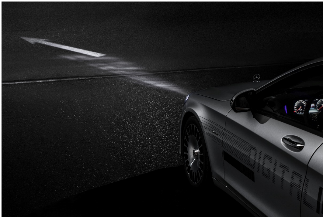
Figure 5. Car projecting a symbol onto the road. The LED matrix makes trailblazing driving assistance possible.
