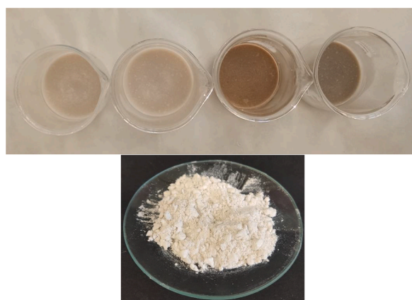
Fig. 7. (a) Image of the glycolysis products obtained from the depolymerization reactions of PET-v, PET-ssp, PET-u and PET-m (from the left to the right) and (b) glycolyzed G-m fraction after purification step.
