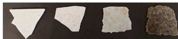
Fig. 6. Images of PET samples obtained by compression molding. From left to right: PET-ssp, PET-v, PET-u and PET-m.
