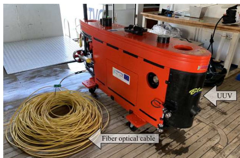
Figure 1. UUV prototype, Blucy, and fiber optical cable during first tests in open sea.
