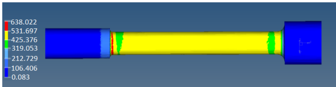
Figure 19. Critical von Mises stress in a headless screw in the 5th metatarsal.
