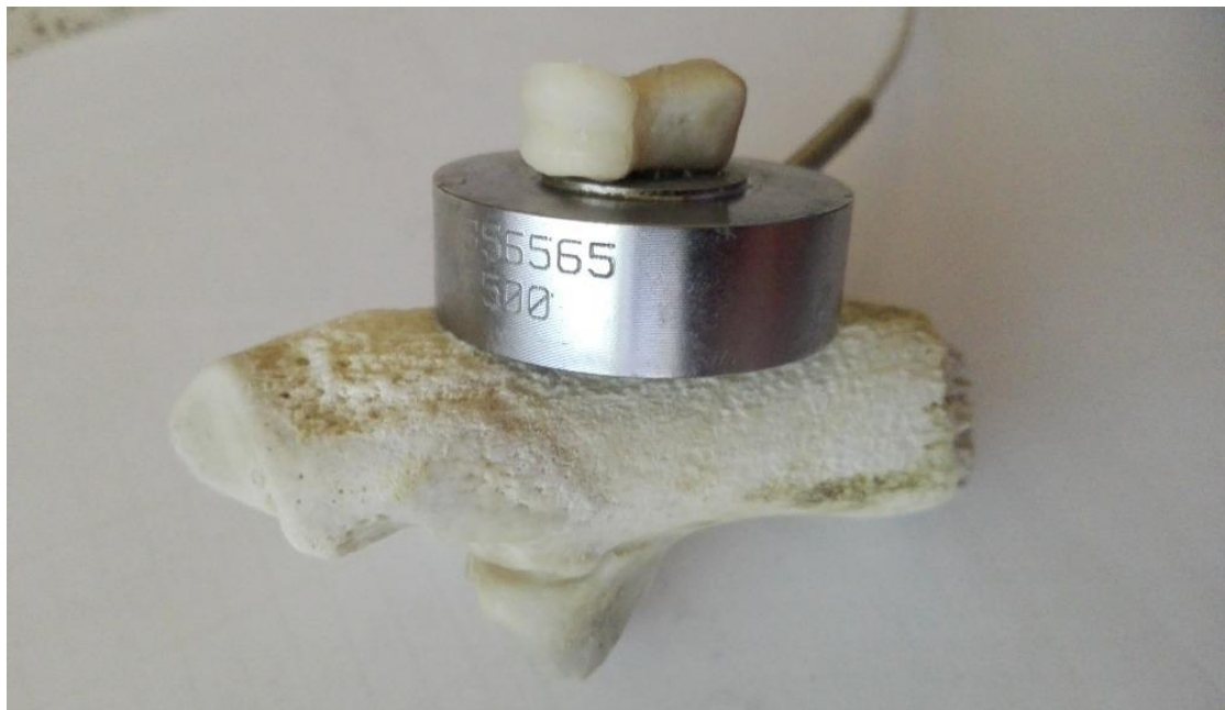
Figure 12. Two bone fragments with a force sensor connected by a headless screw.
