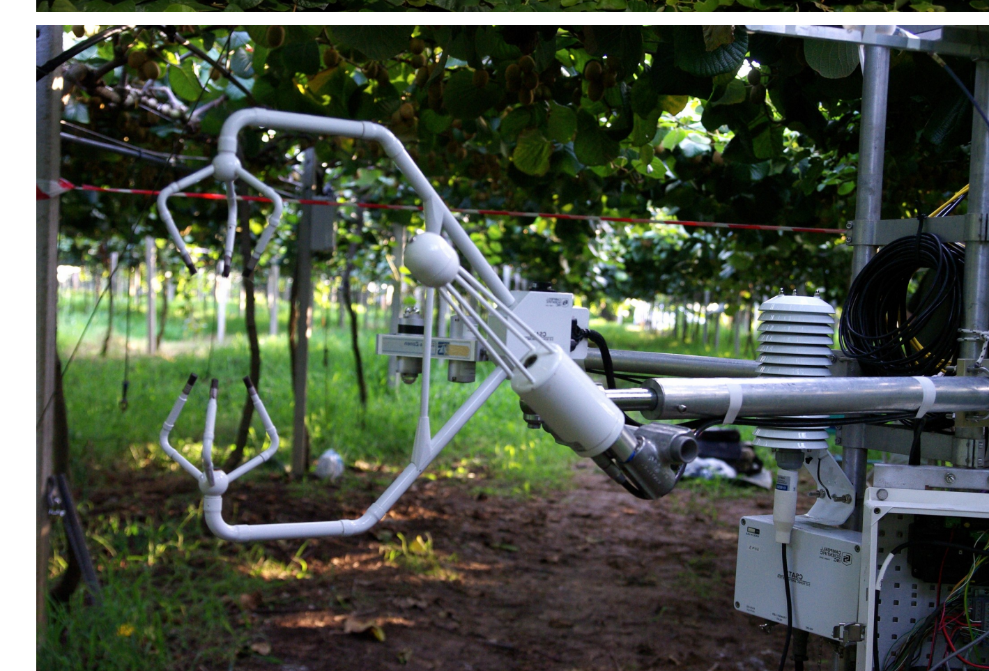
Fig.2: Three aligned eddy covariance systems (sonic anemometers, net radiometers and thermoigrometers) on a vertical mast: above the net, between net and canopies, and below the canopies.
