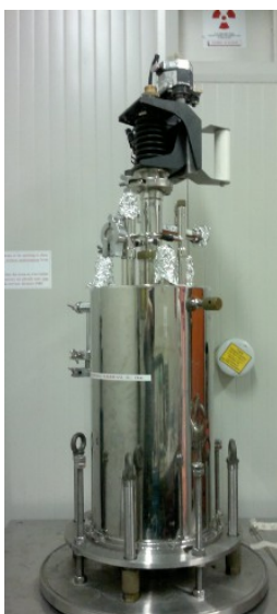
Figure T5: Picture of the cryostat for liquid samples
