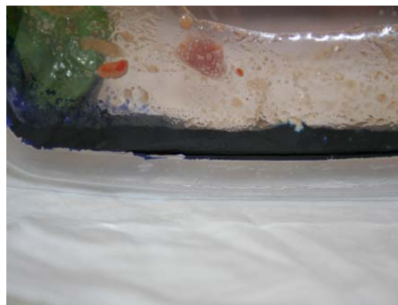
Figure 17 The sealing rubber on this machine was cracked and producing a less than perfect seal.
