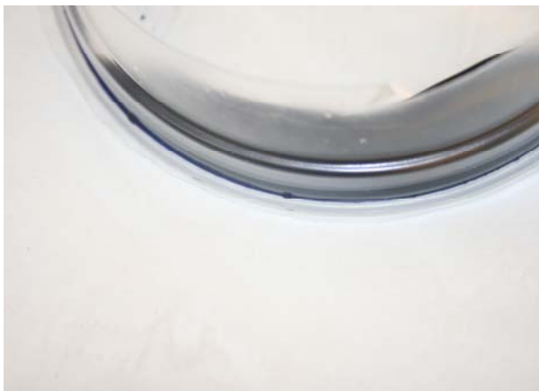
Figure 16 The two notches of blue ink matched exactly the damage seen on the sealing rubber.
