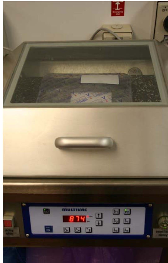
Figure 4 A vacuum test in operation – here with the vacuum at a level of 874mBar. The pack needed to stay inflated for 15 seconds to pass the test. The pack would then be subjected to an increased vacuum to obtain a measure of seal strength.
