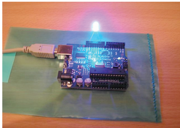
FIGURE 1: Dimitrios Vlastaras' "WebVisitors Blinker." An LED is directly inserted into an Arduino micro-controller. It lights up every time a page of his blog is loaded from the server.
