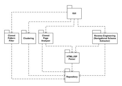
Figure 10 Overall System Architecture
