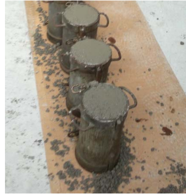
3b.- Cylindrical specimens
