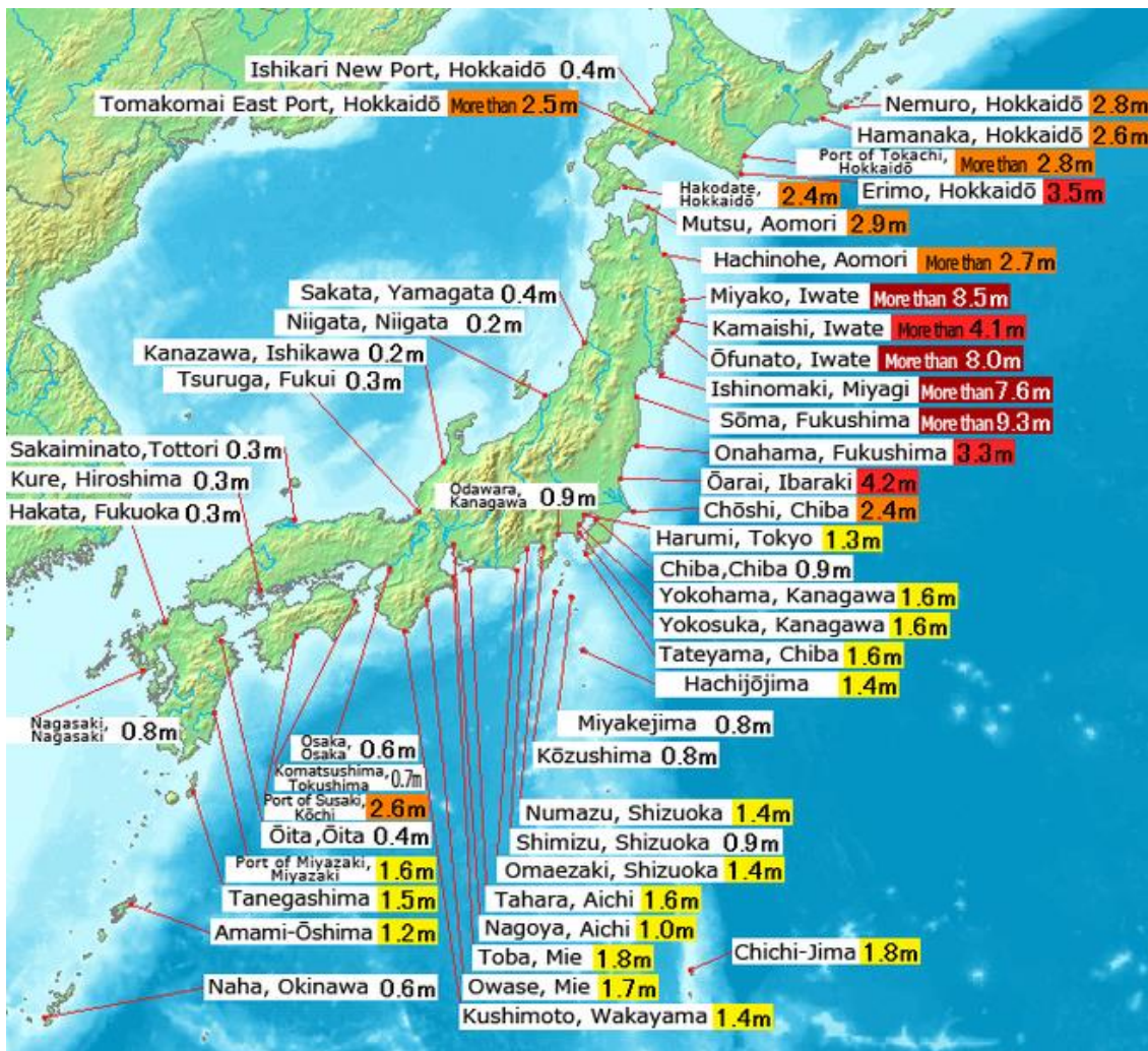
Figure 2 - Tohoku earthquake observed tsunami heights (Wikipedia, 2013a).
