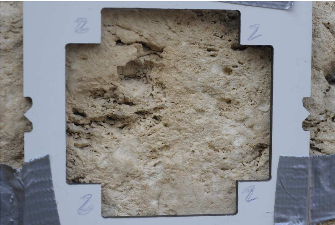
Fig. 6 – "Pietra forte" limestone. This stone is a compact and resistant rock and belongs to the Messinian and also to the Tortonian (i.e., chronostratigraphic units of the Miocene, Cenozoic). Together with "Pietra cantone" stone it has been largely used in the basilica of S. Saturnino, more than all the other lithologies. In the photo it is possible to see the characteristic primary porosity (mainly closed in the matrix) due to the presence of fossils and other elements (Copyright Stefano Columbu and Giorgio Verdiani).
