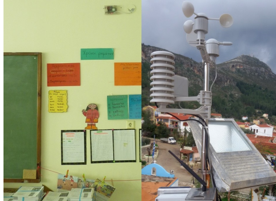
Fig. 1. A close-up of a device installed inside an actual classroom (top of left image) and the weather station used at the Kastelorizo primary school (right image).
