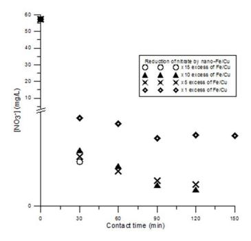
Figure 2: Concentration of residual  $NO_3^-$  in the aqueous solution of NaNO<sub>3</sub> at different Fe<sup>0</sup>/NO<sub>3</sub> weight ratio (initial nitrate concentration 57,25 mg/L; pH – 4,97)
