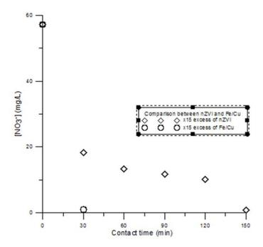
Figure 1: Comparison between nitrate removal by nZVI and nZVI particles coated by Cu (initial nitrate concentration 57,25 mg/L; pH – 4,97)
