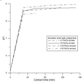
Figure 3: Evolution of pH during the nitrate reduction at different Fe0/NO3- weight ratio
