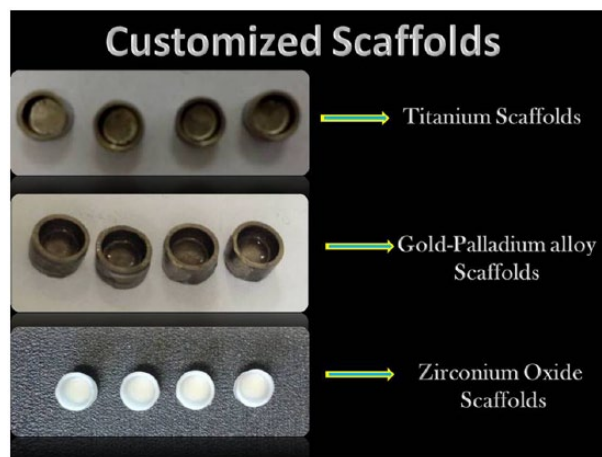
Figure 3. The customized scaffolds. Four titanium samples, four gold–palladium samples, and four zirconia samples.
