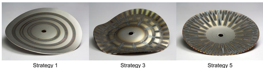
Fig. 10 Achievement of domes by combination of circular and radial scanning patterns (see Table 4 for the laser forming strategies)
