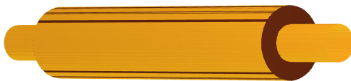
Figure 1: GdfidL model for the azimuthally symmetric beam pipe with resistive insert. The chosen length was L = 30\text{ cm} , the insert thickness a = 5\text{ mm} , the pipe radius plus the insert thickness b = 10\text{ mm} , and the electrical conductivity \sigma_c = 7.69 \cdot 10^5\text{ S/m} for Carbon Fiber Composite (CFC).
