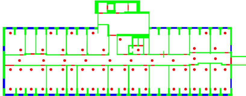
Figure 3. Positions of the N_1 RPs on the Department of Information Engineering, Electronics and Telecommunications (DIET) first floor.
