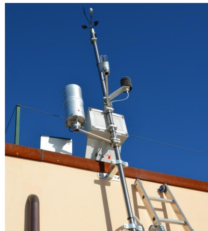
Figure 1. (a) Gravels field overview with albedometer; (b) meteorological sensors.
