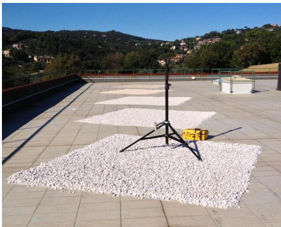
Figure 1. (a) Gravels field overview with albedometer; (b) meteorological sensors.
