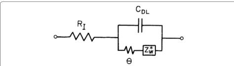
**Fig. 17** Equivalent circtuit of Randles type (adapted from Ho et al. 1980). For symbols explanation, please, refer to Halme et al. (2006)
