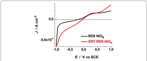
**Fig. 23** Effect of ERY sensitization on the voltammogram of RDS  $NiO_x$  under illumination. Electrolyte: 0.5 M  $LiClO_4$  in propylene carbonate. Electrode is illuminated with white light (intensity: 25 W cm<sup>-2</sup>)
