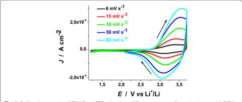
**Fig. 4** Cyclic voltammetries of CS NiO<sub>x</sub> on FTO substrate at different scan rates. Open circuit potential (OCV):  $3.07 \text{ V} \text{ s} \text{ Li}^+\text{/Li}$ . (J current density, E applied potential). Electrolyte as in Fig. 1. *Arrows* indicate the verse of scan
