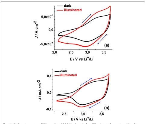
**Fig. 10** Cyclic voltammetry of ERY-sensitised RDS-NiO $_x$  deposited on FTO substrate [scan rate: **a** 12 and **b** 25 mV s<sup>-1</sup>]. OCV: 3.21(dark)/3.24(illuminated) V  $_y$  Li<sup>+</sup>/Li. Radiation source was a halogen white lamp with total intensity of 25 W cm<sup>-2</sup>. *Arrows* indicate the verse of scan
