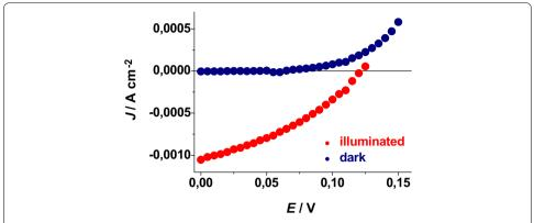
**Fig. 29** JV characteristic curve of the p-DSC with RDS NiO $_x$  deposited onto FTO as photoelectroactive cathode. NiO $_x$  film thickness: 2.5  $\pm$  0.3  $\mu$ m; dye-sensitizer: ERY; solar simulator intensity: 0.1 W cm<sup>-2</sup>.  $\eta$  = 0.045 %;  $V_{\rm CC}$  = 0.120 V;  $J_{\rm SC}$  = 1.05 mA cm<sup>-2</sup>; FF = 36.0 %
