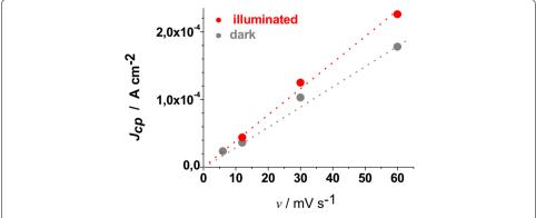
**Fig. 13** Scan rate dependence of the cathodic peaks of ERY-CS NiO<sub>x</sub> in the dark and under illumination. Data are taken from the cyclic voltammetries of Figs. 7 and 11  $(U_{cp})$ : current density in correspondence of the cathodic peak)
