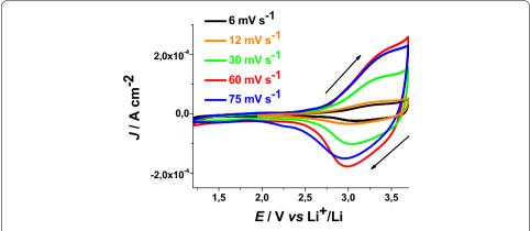
**Fig. 7** Dark cyclic voltammetries of ERY-sensitised CS-NiO $_{\rm x}$  on FTO substrate at different scan rates. *Arrows* indicate the verse of scan
