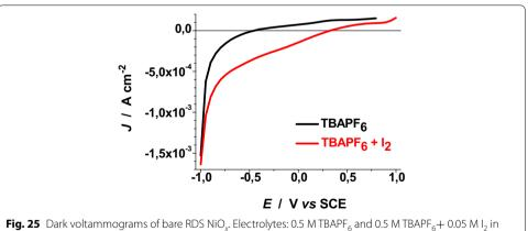
**Fig. 25** Dark voltammograms of bare RDS NiO<sub>x</sub> Electrolytes: 0.5 MTBAPF<sub>6</sub> and 0.5 MTBAPF<sub>6</sub>+ 0.05 M I<sub>2</sub> in propylene carbonate
