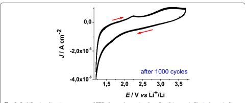
**Fig. 2** Stabilized cyclic voltammogram of FTO after prolonged cycling. Conditions as in Fig. 1. *Arrows* indicate the verse of scan
