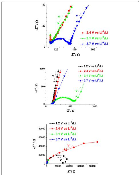
**Fig. 16** Nyquist plots in the high (*upper plot*), medium (*center plot*), and low (*lower plot*) frequency range for CS  $NiO_x$  at 1.2, 2.4, 3.1 and 3.7 V vs  $Li^+/Li$ . Arrows indicate the verse of growing frequencies for the different profiles
