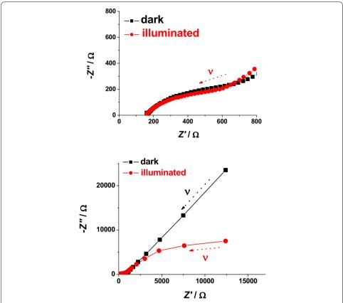
**Fig. 21** Effect of light on the Nyquist plots of ERY sensitized CS  $NiO_x$  polarized at 2.8 V vs Li<sup>+</sup>/Li. High (*upper plot*), and low (*lower plot*) frequency range. *Arrows* indicate the verse of growing frequencies for the different profiles. White light intensity: 22 W cm<sup>-2</sup>
