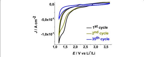
**Fig. 1** Evolution of the voltammogram of uncoated FTO. Electrolyte: 0.7 M LiClO<sub>4</sub> in anhydrous propylene carbonate; counter electrode: Li; reference redox couple: Li $^+$ /Li; scan rate: 5 mV s $^{-1}$ . Open circuit voltage: 2.86 V  $^{\prime}$  S Li $^+$ /Li
