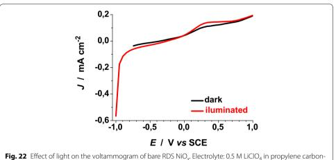
ate. Electrode is illuminated with white light (intensity: 25 W cm<sup>-2</sup>)
