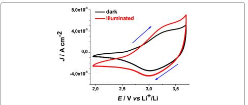
**Fig. 9** Cyclic voltammetry of ERY-sensitised CS-NiO<sub>x</sub> deposited on FTO substrate (scan rate: 12 mV s<sup>-1</sup>). OCV: 3.13(dark)/3.17(illuminated) V vs Li<sup>+</sup>/Li. Radiation source was a halogen white lamp with total intensity of 22 W cm<sup>-2</sup>. *Arrows* indicate the verse of scan
