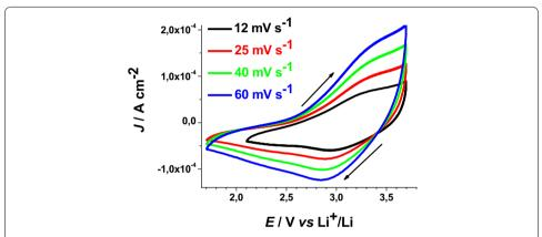
**Fig. 12** Cyclic voltammetries of illuminated ERY-sensitised RDS-NiO $_{\rm x}$  on FTO substrate at different scan rates (incident intensity: 25 W cm $^{-2}$ ). *Arrows* indicate the verse of scan
