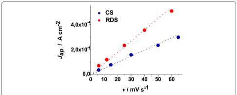
**Fig. 6** Scan rate dependence of the anodic peaks of CS-NiO<sub>x</sub> and RDS-NiO<sub>x</sub> with the same thickness and deposited onto FTO substrate. Data are taken from the cyclic voltammetries of Figs. 4 and 5  $U_{ap}$  current density in correspondence of the anodic peak, v scan rate)
