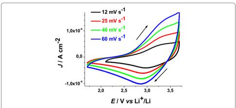
**Fig. 8** Dark cyclic voltammetries of ERY-sensitised RDS-NiO $_x$  on FTO substrate at different scan rates. *Arrows* indicate the verse of scan
