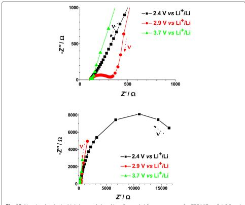
**Fig. 15** Nyquist plots in the high (*upper plot*) and low (*lower plot*) frequency range for RDS  $NiO_x$  at 2.4, 2.9 and 3.7 V vs  $Li^+/Li$ . *Black* and *red arrows* indicate the verse of growing frequencies
