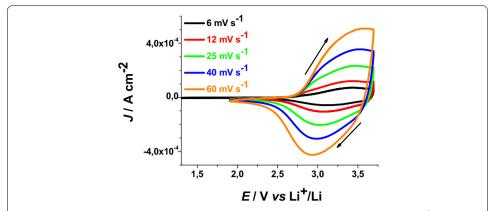
**Fig. 5** Cyclic voltammetries of RDS-NiO<sub>x</sub> on FTO substrate at different scan rates. OCV: 3.24 V vs Li<sup>+</sup>/Li. Electrolyte as in Fig. 1. *Arrows* indicate the verse of scan
