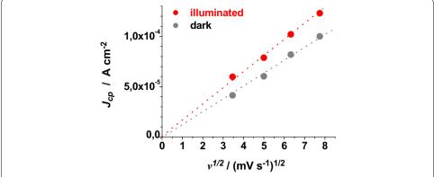
**Fig. 14** Scan rate dependence of the cathodic peaks of ERY-RDS  $\text{NiO}_x$  in the dark and under illumination. Data are taken from the voltammograms of Figs. 8 and 12
