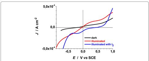
**Fig. 24** Comparison of voltammograms of ERY-RDS  $\mathrm{NiO}_x$  in the dark (*black line*), illuminated with AM 1.5 Solar Simulator with redox species ( $\mathrm{I}_2$ ) in the electrolyte (*green line*), illuminated with AM 1.5 Solar Simulator without redox species (*red line*). Electrolytes: 0.5 M LiClO<sub>4</sub> in propylene carbonate (*red* and *black curve*); 0.5 M LiClO<sub>4</sub> + 0.05 M I<sub>2</sub> in propylene carbonate (*green curve*)
