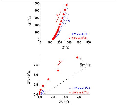
**Fig. 3** Nyquist plots in the high (*upper plot*) and low (*lower plot*) frequency range for FTO at 2.9 V vs Li<sup>+</sup>/Li and 1.2 V vs Li<sup>+</sup>/Li after stabilization of the electrochemical behavior (see Fig. 2). *Blue* and *red full arrows* indicate the verse of growing frequencies. *Black dotted arrows* indicate the point determined at the lowest applied frequency of 5 mHz
