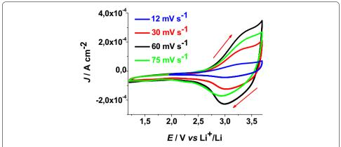
**Fig. 11** Cyclic voltammetries of illuminated ERY-sensitised CS-NiO $_{\rm x}$  on FTO substrate at different scan rates (incident intensity: 22 W cm $^{-2}$ ). *Arrows* indicate the verse of scan
