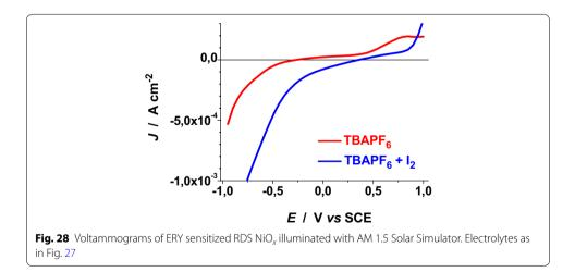
$Ni(II) \rightarrow Ni(III)$  and the reduction process  $NiO_x + n e^- + n Li^+ \rightarrow Li_nNiO_x$ . CS and RDS  $NiO_x$  showed similar electrochemical behaviours with RDS displaying larger current densities of oxidation and possessing a higher number of Ni(III) surface sites with
