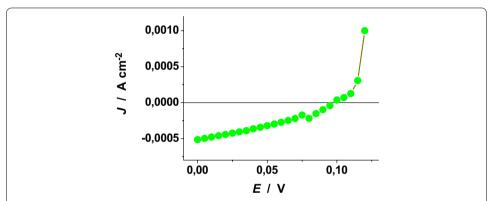
**Fig. 30** JV characteristic curve of the p-DSC with RDS NiO $_x$  deposited onto FTO as photoelectroactive cathode. NiO $_x$  film thickness: 1.5  $\pm$  0.3  $\mu$ m; dye-sensitizer: fast green; solar simulator intensity: 0.1 W cm $^{-2}$ .  $\eta=0.018$  %;  $V_{OC}=0.098$  V;  $J_{SC}=0.51$  mA cm $^{-2}$ ; FF = 36.7 %
