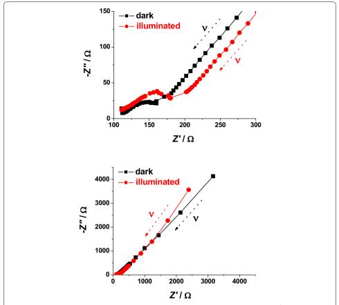
**Fig. 20** Effect of light on the Nyquist plots of ERY sensitized RDS  $\mathrm{NiO}_x$  polarized at 2.9 V vs Li<sup>+</sup>/Li. High (upper plot), and low (lower plot) frequency range. Arrows indicate the verse of growing frequencies for the different profiles. White light intensity: 25 W cm<sup>-2</sup>
