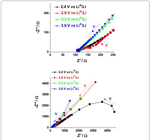
**Fig. 19** Nyquist plots in the high (*upper plot*), and low (*lower plot*) frequency range for ERY sensitized RDS  $NiO_x$  at 2.4, 2.9, 3.3 and 3.6 V vs  $Li^+/Li$ . Arrows indicate the verse of growing frequencies for the different profiles
