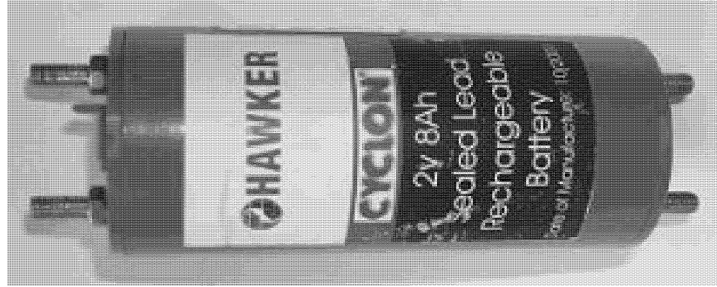
Fig. 2: 8Ah sealed lead-acid test cell
