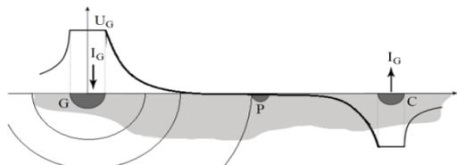
Figure 2. Potential profile between the ground electrode G and the auxiliary current electrode C.
