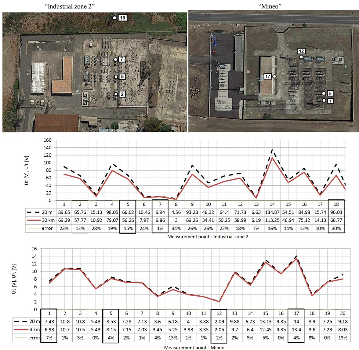
Figure 8 Touch voltage measurements done in the 150/20kV substations “Industrial Zone 2” and “Mineo” (Catania, Sicily, Italy) with the auxiliary current electrode located at 20 m from the grounding system contour (dashed line in the graph) and at 30 km and 3 km respectively (continuous line in the graph). (Performer: Technician Emanuele Falanchi, Enel, Italy).
