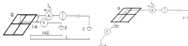
Figure 3. Methods  $0^\circ$  and  $90^\circ$  of impedance measurement in a grounding system.
