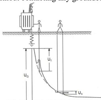
Figure 1. The ground potential rise (GPR)  $U_G$ , the touch voltage  $U_t$  and the step voltage  $U_s$ .
