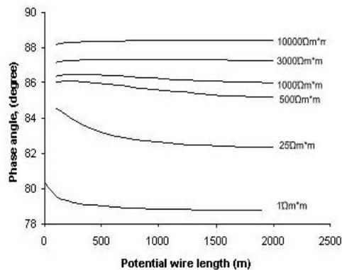
Figure 5. Phase angle  $\varphi_{CE}$  in dependence of the potential wire lengths and the soil resistivity for impedance of the coupling effect
