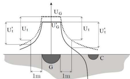
Figure 6. Potential behaviors of a hemispherical electrode with a single C current electrode at remote point (dashed line) and at short distance (continuous line).
