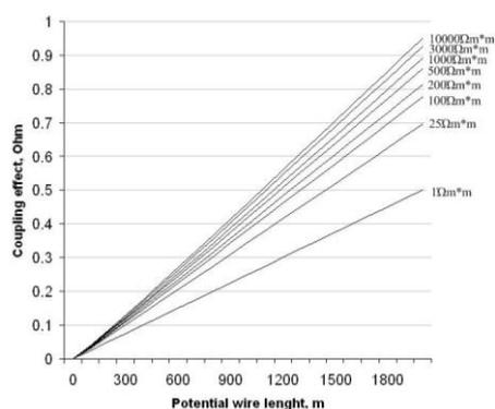
Figure 4. Curves of coupling effect  $Z_{CE}$  (as impedance amplitude) versus potential wire length up to 2,000 m and different soil resistivity
