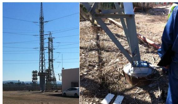
Figure 7. Conservative touch voltage  $U_t$  tests done on a line tower footing installed in a corner of HV/MV substation in Kyriat, Israel (Technical team of IEC R&D Lab. Haifa)
