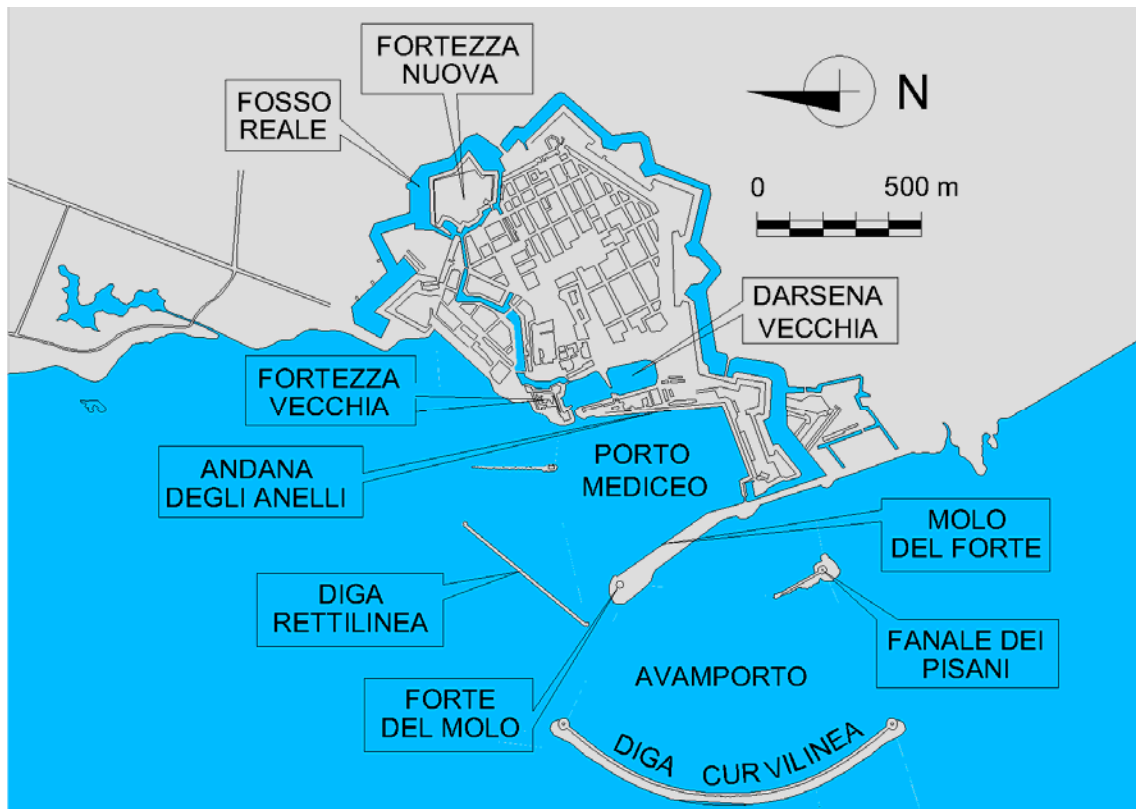
Fig. 6 Project of the Diga Curvilinea (curvilinear breakwater) and of the Diga Rettilinea (straight breakwater) of the Poirel (1851).
