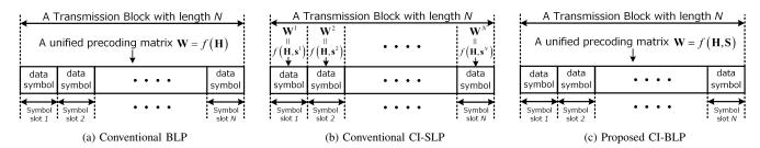
Fig. 1: A comparison between different precoding methodologies
