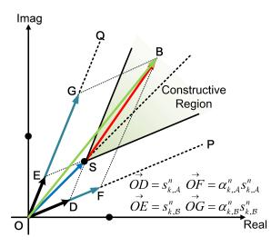
Fig. 2: An illustration for CI, 8PSK, 'symbol-scaling' metric
