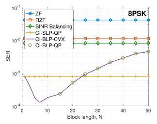
Fig. 10: SER v.s. block length N, 8PSK,  $N_{\rm T} = K = 12$ , SNR = 30dB
