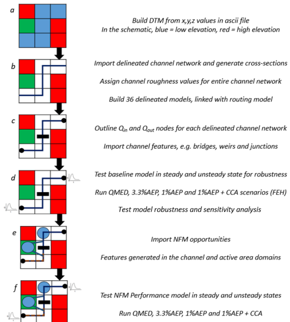
Figure 3. Model build schematic example for one of the sub-catchment models. Coloured squares represent elevation, blue (low)—green (middle)—red (high). Blue circles conceptually represent NFM features, and the black line across the channel is an in-channel feature (e.g., bridge).
