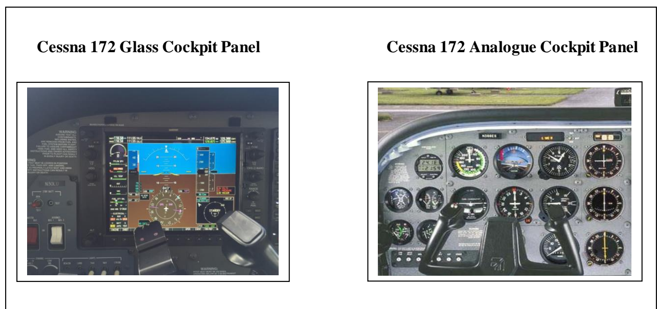
Figure 1 Cessna 172 Glass vs Analogue Cockpit Panel
