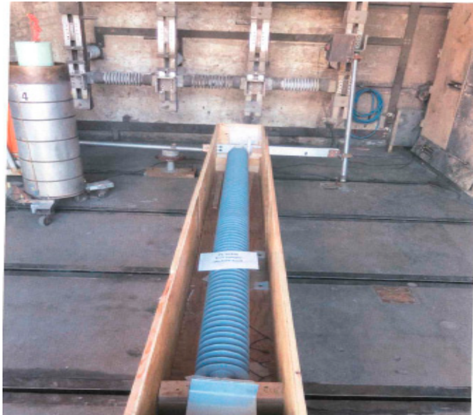
Figure 6. Laboratory set-up of a 132 kV NCIT.
