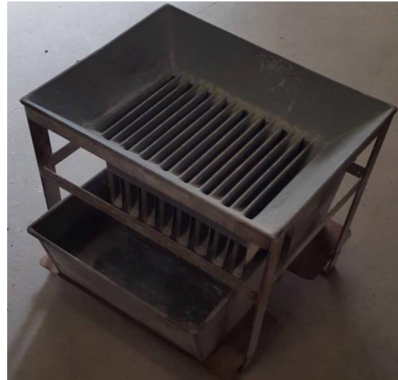
Figure 4. Riffle splitter used to separate the material into equal portions
