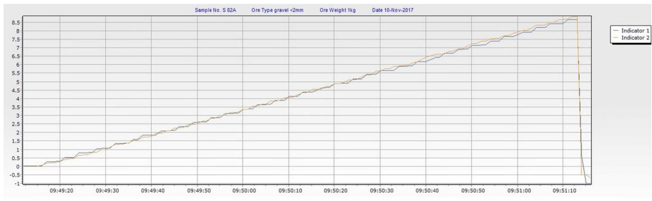
Fig. 10 Gravel 2 mm particle size. Breakfree force test sample 1000 g. Water added to the bucket at 2 l per minute
