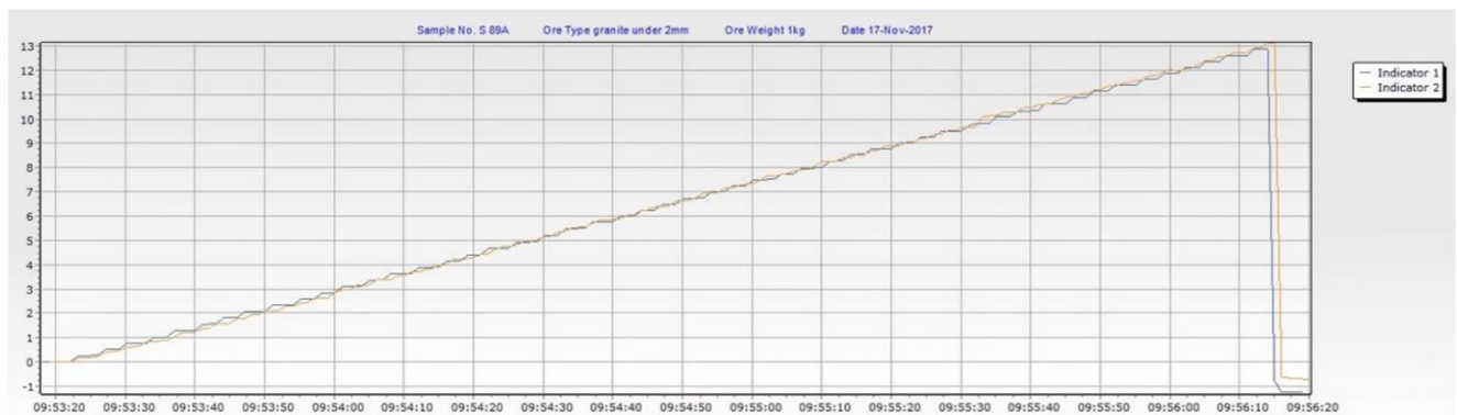
Fig. 11 Granite 2 mm particle size. Breakfree force test sample 1000 g. Water added to the bucket at 2 l per minute
