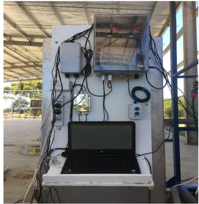
Fig. 9 Test Rig 1. Instrumentation and load cell displays
