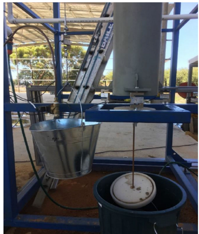
Fig. 7 Test Rig 1, ore tube open
