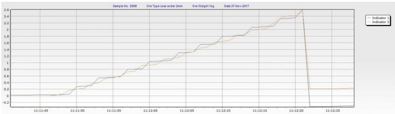
Fig. 12 Coal 2 mm particle size. Breakfree force test sample 1000 g. Water added to the bucket at 2 l per minute
