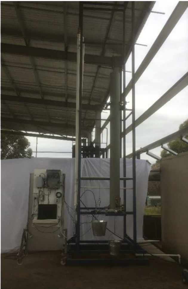
Fig. 8 Test Rig 1. Constant water head flow pipe (white pipe)
